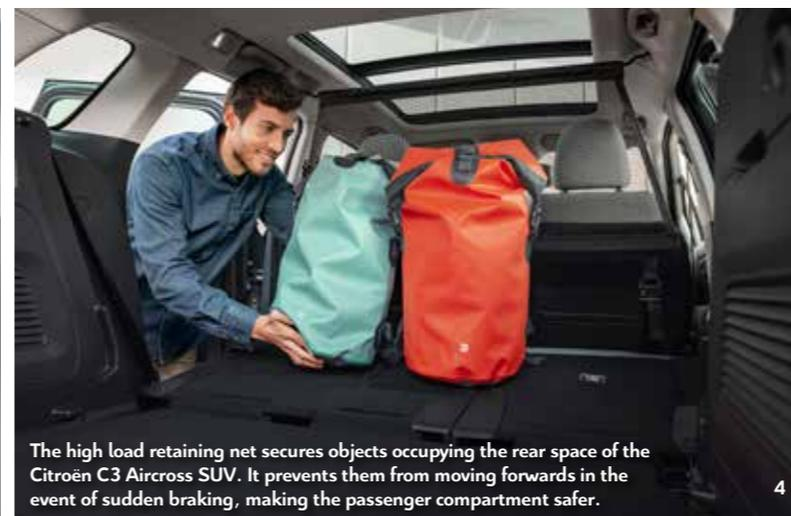
The high load retaining net secures objects occupying the rear space of the Citroën C3 Aircross SUV. It prevents them from moving forwards in the event of sudden braking, making the passenger compartment safer.
